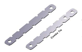
Aluminum form ties secure aluminum forms in order to pour the desired wall thickness. These ties are used predominantly for poured wall basement foundations around the country.
