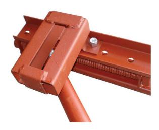
OCM, Inc's Bridge Overhang Bracket Guard Rail Receptacle is made to allow the placement of guardrail posts on exterior framework. The Bridge Overhang Bracket Guard Rail Receptacle attaches securely to the Bridge Overhang Bracket Extension and accepts 2x4 guardrail posts.
