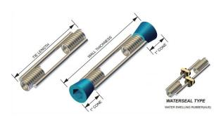
OCM Conefast Coil Ties are one of the most economical and versatile form tie systems available. They are commonly used with self cleaning Coil Rod or Coil Bolts. The Conefast coil Ties have extended coils that protrude beyond the end of the struts allowing for a Conefast (Screw On) Cone to be attached.
