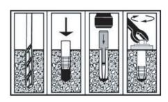
OCM Coil Thread Drop In Anchors are internally threaded Drop In Expansion Anchors used with either 1/2" or 3/4" Diameter Coil Rod, and are set in place by the use of the Setting Tool after the anchor is placed into the properly sized pre-drilled hole.
