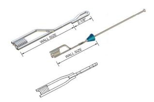
OCM Combo Ties are manufactured with either a Standard Loop Tie or Snap Tie on one end and a 1/2" Coil Tie on the other end. They can be used in Steel Frame Form or Snap Tie one sided or blind side forming applications.
