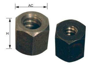
OCM Tall Coil Nuts are made from high strength steel, and are used with different types of coil thread bolts and rods in concrete formwork, bridge deck forming, or precast concrete applications.
