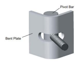
OCM Weld Angle Brackets are designed to tie one-sided forming to steel piles, metal beams, weld plates, etc. The pivot pin is furnished with Coil Thread or Euro Thread. The OCM Weld Angle Bracket allows the form tie a pivot range of 110° (55° each direction), and will exceed the tensile capacity of the form tie when properly installed by a certified welder.
