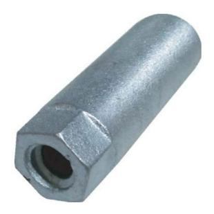
OCM, Inc's Euro Rod Round Nuts w/ Hex End is made of high strength steel. The metric thread provides for a fast threading connection with 15mm Euro Rod. The increased length ensures maximum thread engagement.
