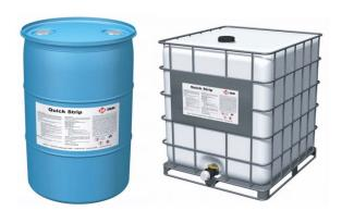
A quality, chemically-neutral, petroleum based form release agent. OCM Quick Strip reacts with the alkali in the concrete to form a soap film that inhibits the bonding of fresh concrete to the formwork. Forms are ready for re use almost instantly. OCM Quick Strip produces a smooth, void free, architectural concrete surface. VOC compliant.
