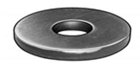
OCM Neoprene Washers are designed to be tight fitting around the circumference of OCM Coil Rod and/or OCM Euro Rod. Neoprene washers are tight fitting, and are typically positioned near the center of a tie. Neoprene Washers are used to to resist water seepage along the tie by breaking the surface continuity of the wire.
