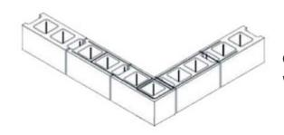
OCM, Inc's Masonry Wire Fabricated Corners are used with Masonry Wire Ladder around 90 degree turns.
