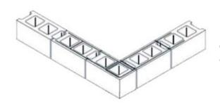
OCM, Inc's Masonry Wire Fabricated Corners are used with Masonry Wire Ladder around 90 degree turns.
