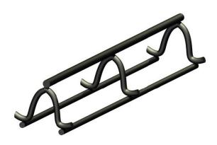
OCM Slab Bolster Upper (Commercial Grade) metal bar supports are used in commercial concrete projects to support upper and lower mats of reinforcing steel in elevated concrete decks, footings, slab on grade, slab on metal deck, bridge decks and other applications.
