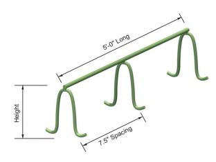
OCM Continuous High Chair Epoxy Coated metal bar supports are used in commercial concrete projects to support upper and lower mats of reinforcing steel in elevated concrete decks, footings, slab on grade, slab on metal deck, bridge decks and other applications.
