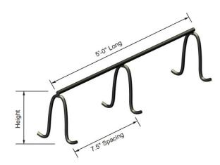
OCM Continuous High Chair metal bar supports are used in commercial concrete projects to support reinforcing steel in elevated concrete decks, footings, slab on metal deck, bridge decks and other applications.
