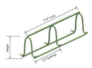
OCM Continuous High Chair Upper Epoxy Coated metal bar supports are used in commercial concrete projects to support upper and lower mats of reinforcing steel in elevated concrete decks, footings, slab on grade, slab on metal deck, bridge decks and other applications.
