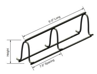
OCM Continuous High Chair Upper metal bar supports are used in commercial concrete projects to support reinforcing steel in elevated concrete decks, footings, slab on metal deck, bridge decks and other applications.
