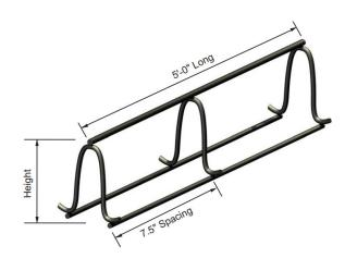
OCM Continuous High Chair Upper metal bar supports are used in commercial concrete projects to support reinforcing steel in elevated concrete decks, footings, slab on metal deck, bridge decks and other applications.
