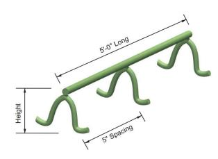
OCM Slab Bolster Epoxy Coated metal bar supports are used in commercial concrete projects to support upper and lower mats of reinforcing steel in elevated concrete decks, footings, slab on grade, slab on metal deck, bridge decks and other applications.
