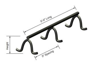
OCM Slab Bolster (Commercial Grade) metal bar supports are used in commercial concrete projects to support reinforcing steel in elevated concrete decks, footings, slab on metal deck, bridge decks and other applications.
