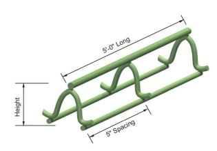
OCM Slab Bolster Upper Epoxy Coated metal bar supports are used in commercial concrete projects to support upper and lower mats of reinforcing steel in elevated concrete decks, footings, slab on grade, slab on metal deck, bridge decks and other applications.
