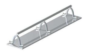
OCM Slab Bolster with Plate are used in commercial concrete projects to support lower mats of reinforcing steel in footings, slab on grade on soil, rock or sand conditions.
