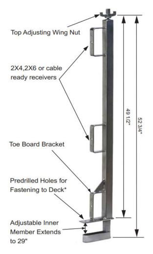
OCM, Inc's Heavy Duty Slab Grabber are used as guardrails that are fast, easy, and affordable. Made from high-strength galvanized steel; capable of withstanding at least 200 lbs. The Heavy Duty Slab Grabber meets FEDERAL OSHA 1926 502(B)(3) requirements.
