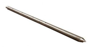
OCM Premium D Steel Stakes with holes are primarily used to secure wood or metal forms to the grade in flatwork applications. Other uses may include attaching screed bar holder clamps in flatwork finishing, securing landscape timbers, surveying stakes, string line guides, securing metal forms with pockets and securing wood forming for flatwork.
