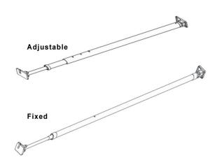
OCM, Inc's Pipe Braces are used for formwork, precast, and tilt-up bracing applications. Choose from 3 types of pipe braces; standard, heavy duty, and long heavy duty.
