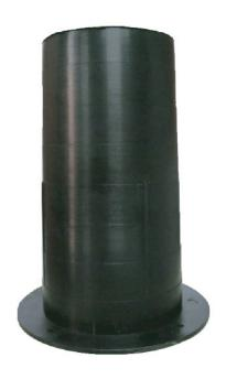
OCM, Incs Concrete Sleeves are used commonly on high rise structures to create a vertical pass through void for piping and conduit. They are injection molded from high strength, yet flexible, polyethylene. They save labor because they are tapered and can easily be removed after the forms have been stripped. OCM Concrete Sleeves may be telescoped or cut to accommodate any slab thickness and are easy to cut with a utility knife.
