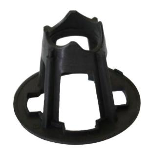
OCM Polymer Composite Cradle Chair may be used to support mesh or rebar in many applications requiring heavy load capacity. Common applications include slab on grade, insulated sandwich panels, vapor barrier, and on poorly compacted or loose soils. OCM Polymer Composite Cradle Chairs meet current CRSI requirements.
