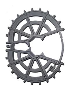
The OCM Locking Wheel Spacer is a polymer composite bar support used to maintain the position of rebar during placement and is typically used in lateral positioning applications. It can be used to position vertical rebar from the side forms.
