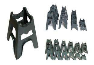
OCM, Inc's Pro Chairs are made with high performance, high strength polymer composite material that won't rust. The cradle shaped head will provide aid in positioning rebar. The 2-in-1 cradle head allows for one Pro Chair to be used for two different heights, reducing the amount of inventory you need to take on.
