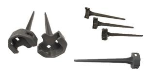
The Polymer Composite Stud Chair snaps on to the head of the stud of an embed plate in tilt-up and precast panels to set the embed plates at the correct height.
