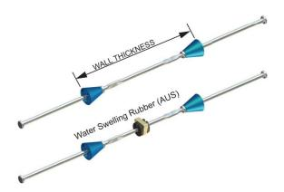
OCM High Strength Bay Ties are manufactured with 1/2" Hex Heads and Plastic Form Spreaders. OCM High Strength Bay Ties provide a safe working load of 3500 lbs. with an average ultimate load of 7000 lbs. OCM High Strength Bay Ties are designed to easily tie lumber forming systems.
