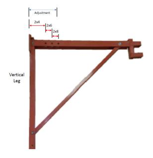
OCM SBRACT-A90 Scaffold Bracket supports scaffolding with many forming systems. OCM's Scaffold Bracket is easily adjusted to accommodate varying waler thicknesses by positioning the vertical leg on the horizontal channel.
