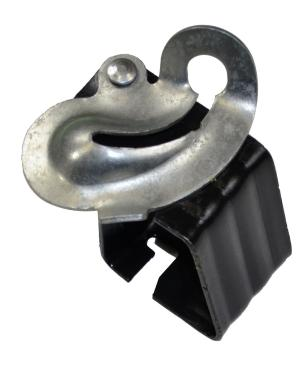
The A Clamp is a holding device fabricated from high strength steel that is used in a single waler snap tie forming application to ensure proper load distribution when installed correctly. A Clamps work with Short End Snap Ties, single horizontal walers, or single vertical strongbacks. The A Clamp Body is set against the waler or stiffback and the clamp rotates across the tie just inside the tie head drawing up all of the components until snug.
