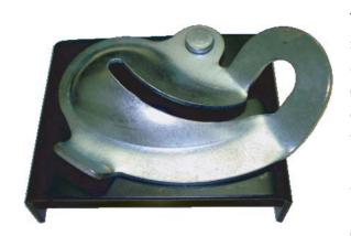
The C Clamp is a holding device fabricated from high strength steel that is used in snap tie forming applications that is designed to ensure proper load distribution when installed correctly. C Clamps work in conjunction with Long End Snap Ties, double horizontal walers and double vertical strongbacks. The C Clamp Body is set against the outer double vertical strongbacks and the face of the clamp rotates across the tie just inside the tie head drawing up all of the form components until snug.
