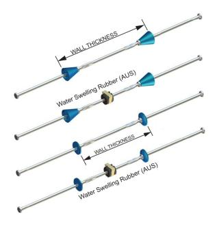
OCM Heavy Duty Snap Ties are manufactured with integral heads, and Metal or Plastic Form Spreaders. OCM Heavy Duty Snap Ties are designed to easily tie lumber forming systems. OCM Heavy Duty Snap Ties have a nominal 1" breakback. Each Tie incorporates an anti-turn device in order to properly break after use.
