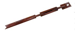
OCM, Inc's Turnbuckle Heavy Duty are form aligners that accurately position and plumb vertical forms. The Turnbuckle Heavy Duty has a 1" diameter coil that is self-cleaning for fast adjustments. It features a bent plate with nail holes and a 15/16" hole that fits 3/4" or 7/8" steel stakes.
