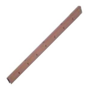
OCM, Inc's Metal Filler are made from cold formed ushape sections and are available in 1", 1-1/2", and 2" width (available in 9FT upon request). Metal Fillers are compatible with other handset steel/plywood forming systems, and are used to attach two panels, or a panel and a corner of the poured wall.
